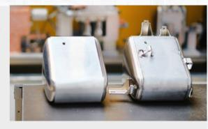
The area of aluminum welding is completed by our automated helium leak testing systems, which guarantee excellent product quality.
