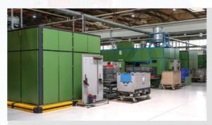
All products manufactured by JAHN GmbH are cleaned in modern solvent washing systems. In our efficient facilities, all manufactured products are reliably and cleanly degreased in this way. Existing cooling lubricants are completely removed in this process in order to deliver a high-purity aluminium product.
