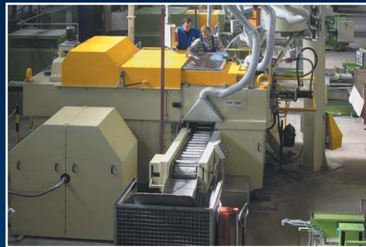
impact extrusion on toggle lever press
