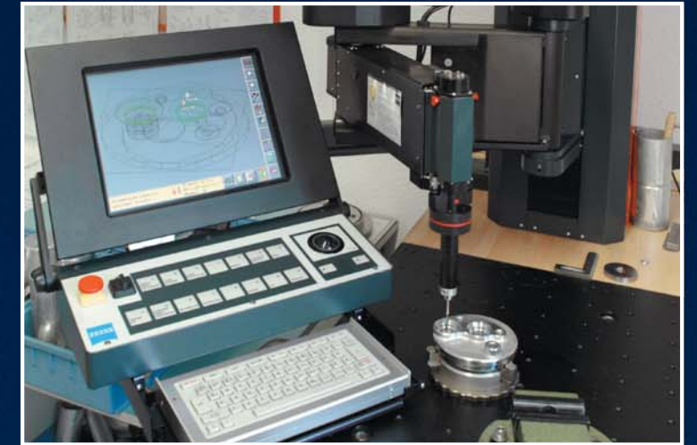
complex measuring and inspection machine
